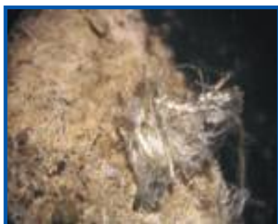
Chrysotile (white asbestos) in asbestos cement roof sheet
