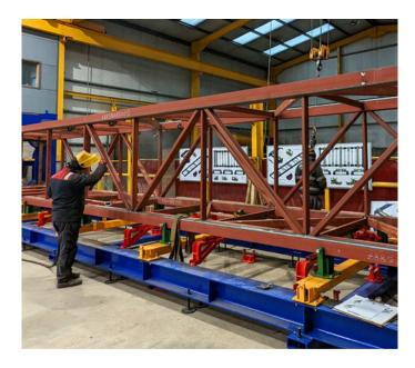
To facilitate the precision fabrication of these sections, a custom-engineered jig—measuring approximately 15 meters in length—was designed and manufactured.
